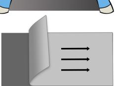
Note: The Privacy Filter is to be installed matte side out.
