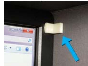
Image 5 Support bracket placement, actual brackets are black.
